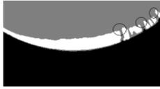
Fig.12 Discontinuous wear lands and abnormal cusps of the inner-contour
