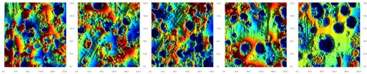
(a) After conditioning (b) 5minute polishing (c) 10minute polishing (d) 15minute polishing (e) 30minute polishing
