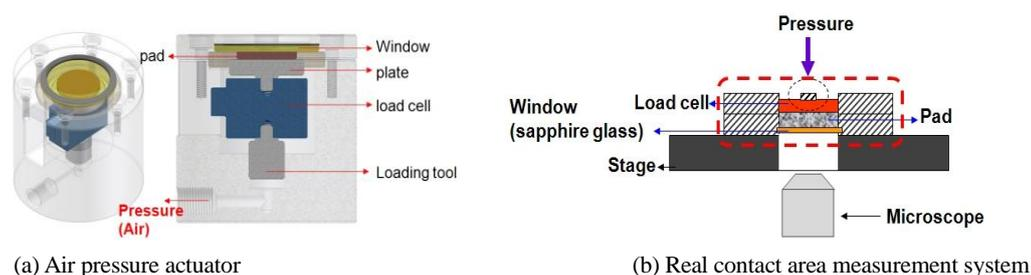
Fig. 1 Schematic of real contact area actuator and system
