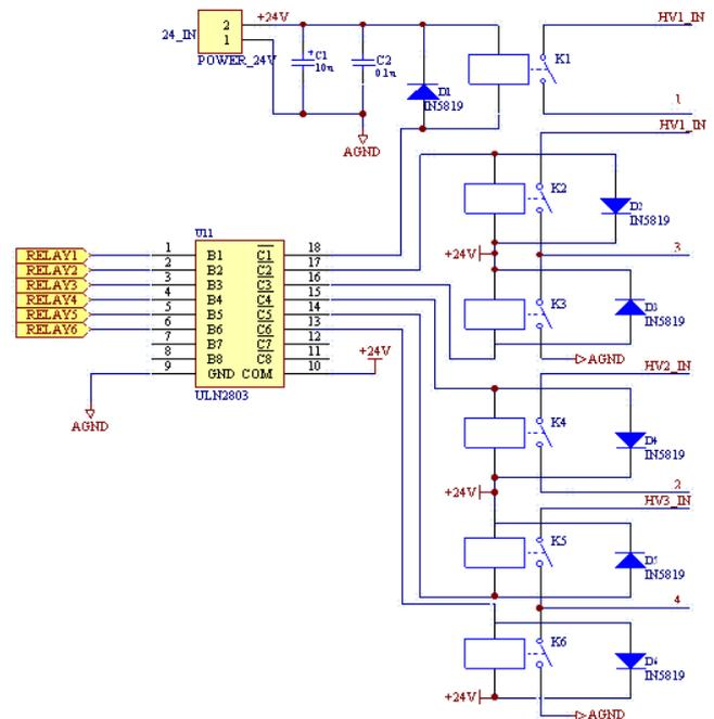
Fig. 3 Circuit diagram of the relay array.
