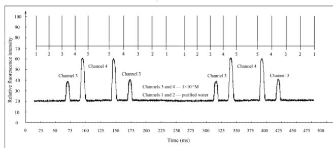
Fig. 10 Typical electropherograms of separation of samples. Channels 1, 2 and 3, 4 were filled with purified water and Rhodamine B sample ( $1.0 \times 10^{-4}$  mol/L). The volume of sample in channel 4 was larger than its in channel 3. Analytical conditions: 10m mol/L  $\text{Na}_2\text{B}_4\text{O}_7$  running buffer; the sample loading operation of 600 V for 20 s; the separation voltage of 800 V.
