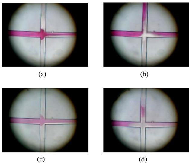
Fig. 8 Effect of injection process (a, c) and separation process (b, d) in different conditions (a, b is under the circumstance of improper voltage ratios and c, d is in the condition of proper voltage ratios) for the cross-shaped capillary electrophoresis microchip.
