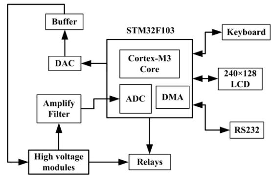
Fig. 2 Block diagram of overall system structure showing the components and their correlation.
