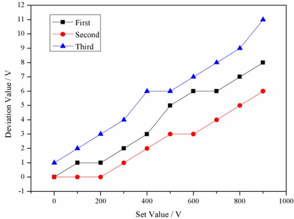
Fig. 6 Comparison between set value and deviation value of each route of high-voltage power supply.
