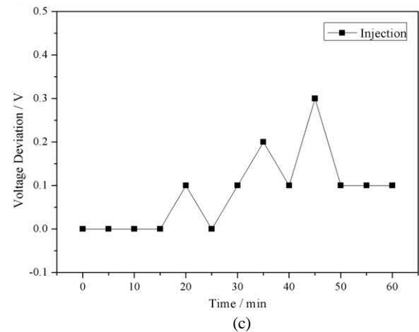
Fig. 7 Time shift characteristic of high-voltage power supply including (a) the first route, (b) the second route and (c) the third route.
