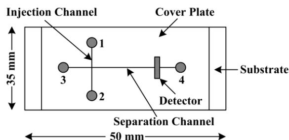
Fig. 5 Layout of the cross-shaped capillary electrophoresis microchip, comprising an injection channel and a variable length separation channel: 1 sample inlet, 2 sample outlet, 3 buffer inlet, and 4 buffer outlet.
