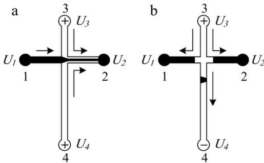
Fig. 1 Typical electrophoresis principle in the microfluidic chip composed by (a) sample injection and (b) sample separation.
