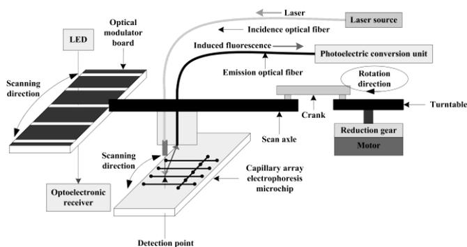
Fig. 9 Schematic diagram of multichannel detection structure comprising laser induced fluorescence detection subsystem, channel identification unit and fluorescent signal processing subsystem.
