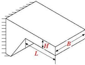
Fig.1 Structure of the microcantilever
