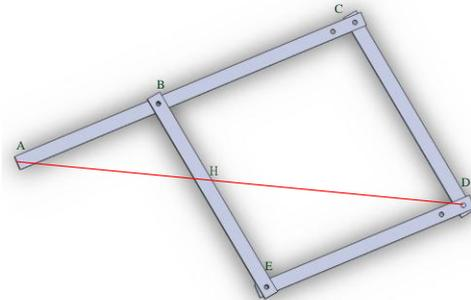
Fig.3 Pantograph mechanism
