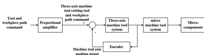
Fig.9 Schematic diagram of open-loop control system
