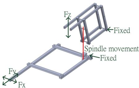
Fig.2 Pantograph based micro-platform
