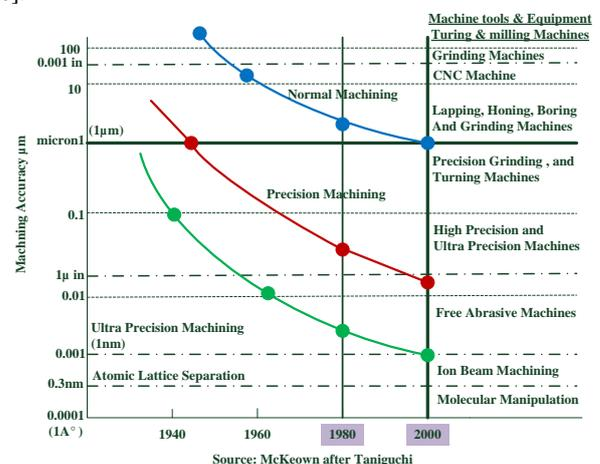
Fig.1 Micromachining capability over time[1].
