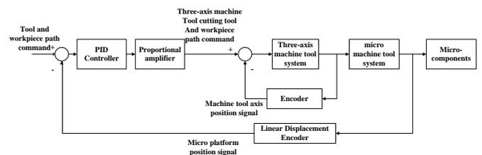
Fig.11 Schematic diagram of closed-loop control system
