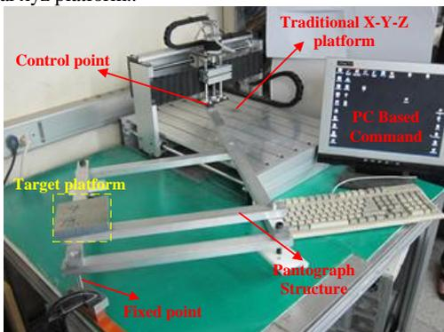
Fig.8 Prototype of Micro-Machining Machine
